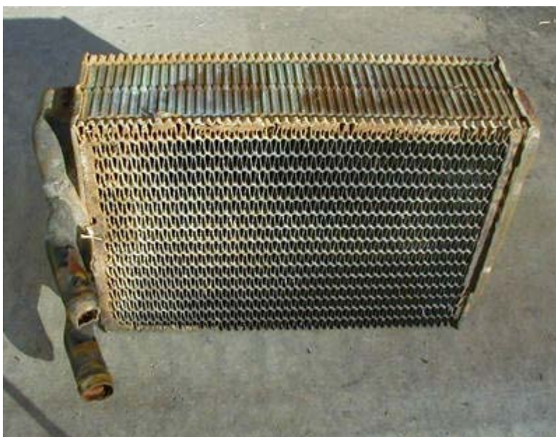
A heater core looks like a small radiator.
